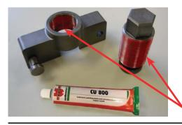
Apply copper anti-seize to rod and top block threads
