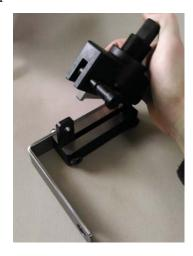
**Step 2:** Place belt cutter jaws around elevator belt.
